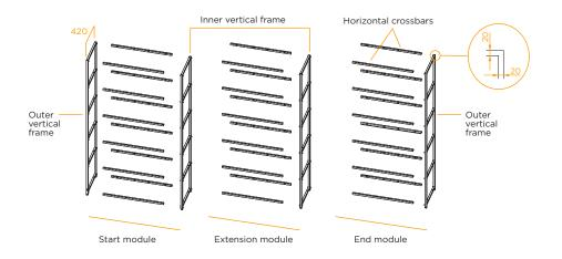
The steel profiles are degreased, washed and phosphated before being coated with  $60/80\mu m$  epoxy powder and then polymerised. The powder coating complies with the current reaction to fire standard UNE 23827-90.
